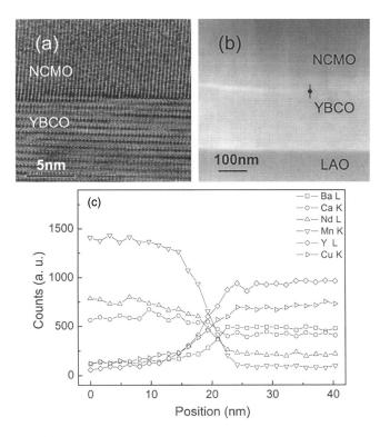
FIG. 1. (a) High resolution TEM image of N/Y(2) at the interface, (b) image of HAADF of NCMO/YBCO/LAO cross section, and (c) profile of EDS across the NCMO/YBCO interface. The vertical line indicates the path of scanning within 40 nm.
