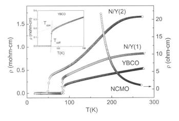
FIG. 2. Resistivity ( $\rho$ ) vs temperature (*T*) for NCMO with the right scale and YBCO, N/Y(1), and N/Y(2) with left scale. The arrows indicate the positions of  $T_{\rm con}$  and  $T_{\rm coff}$  in the inset.
